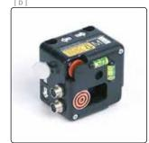
Measuring unit M, 2 axis, PSD 18x18 mm, inclinometer (Discontinued)
